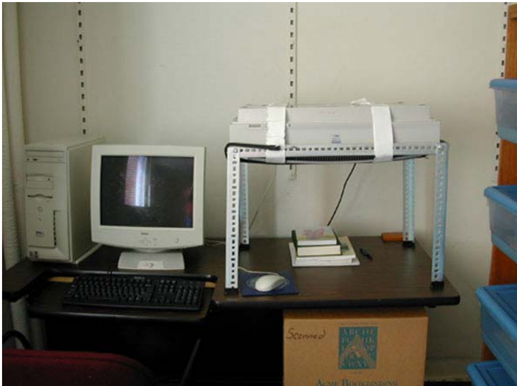
Fig. 1. Specimen scanning workstation showing inverted scanner and custom-built stand
